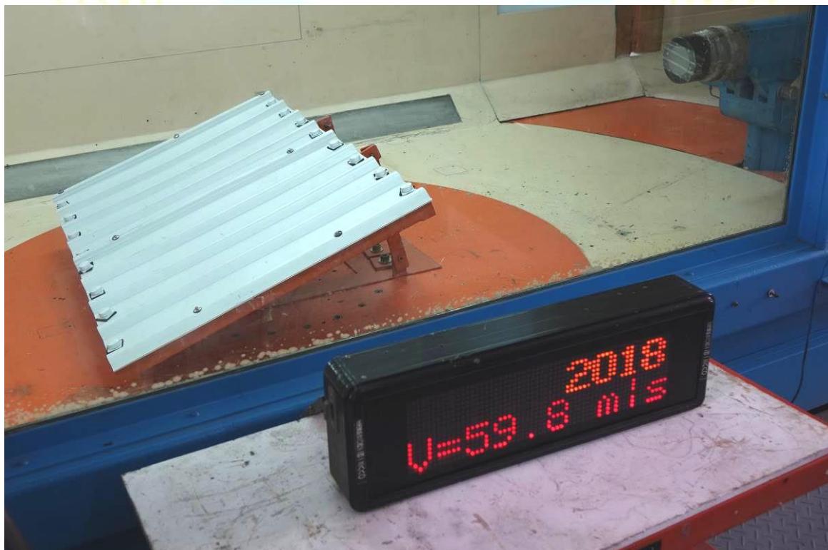
Figure. 4 The Corrugated Foam Sheet is under the test, V = 59.8 \text{ m/s}
