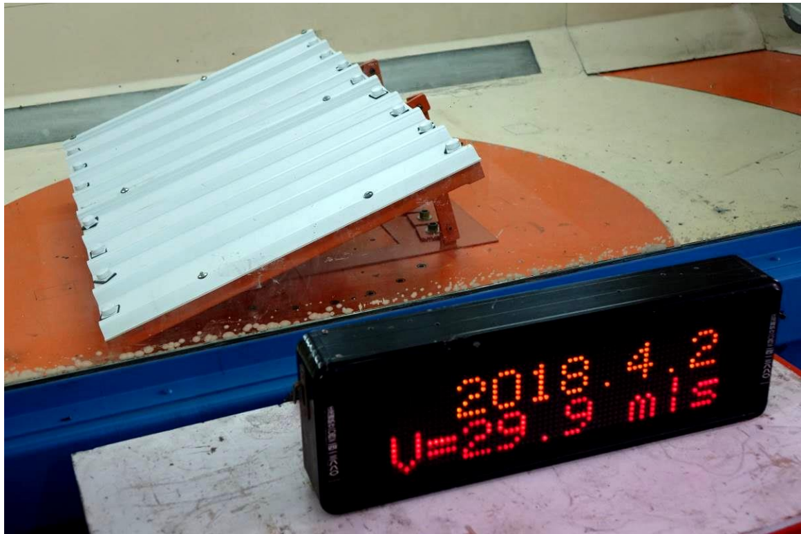
Figure. 3 The Corrugated Foam Sheet is under the test, V = 29.9 \text{ m/s}
