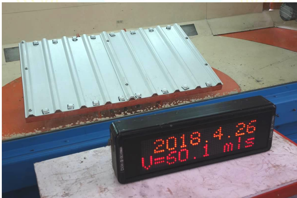
Figure. 10 The Corrugated Foam Sheet is under the test, V = 60.1 \text{ m/s}
