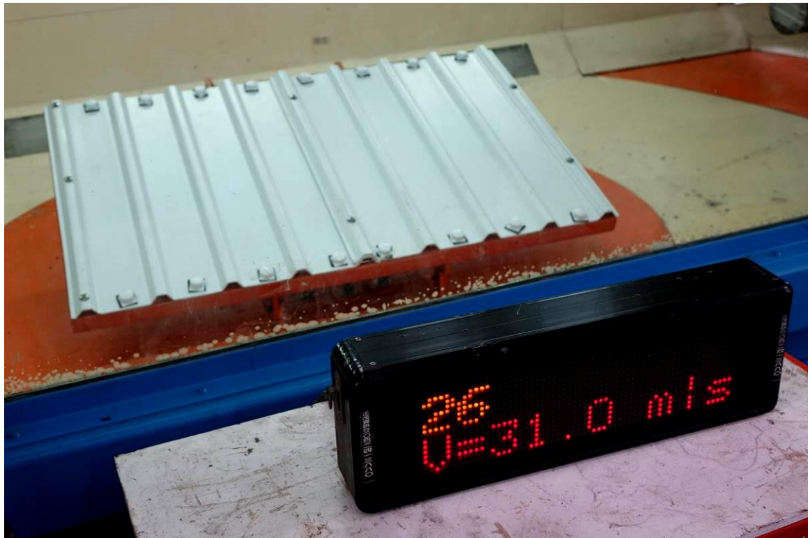
Figure. 9 The Corrugated Foam Sheet is under the test, V = 31.0 \text{ m/s}
